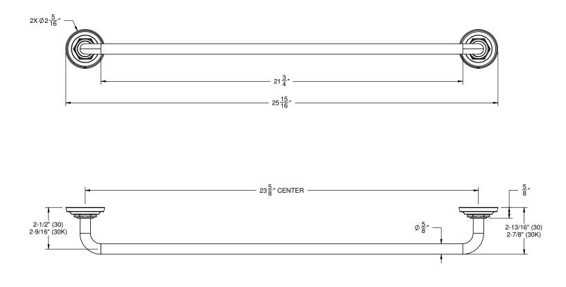
(4X) 8 x 1-1/2" PHILLIPS HEAD SCREW (4X) 3/8" - 1/2" WALL ANCHOR ALL DIMENSIONS SHOWN TO NEAREST 1/16"
