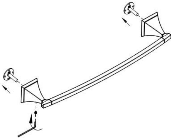
② ALIGN MOUNTING BRACKETS AND MARK LOCATION
