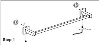
Loosen the set screw on the accessory and remove the backing plates. Position the accessory against the wall and mark outline with pencil.
