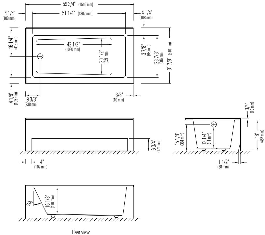
\*A bathtub fitted with back jets can cause the pump to protrude by approximately 3" from the overall dimension.
