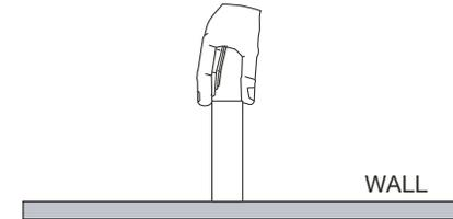
2. Using the Allen key provided, remove the mounting post from the ring post. Press the mounting post against ring post position on the wall and mark the screw hole positions.
